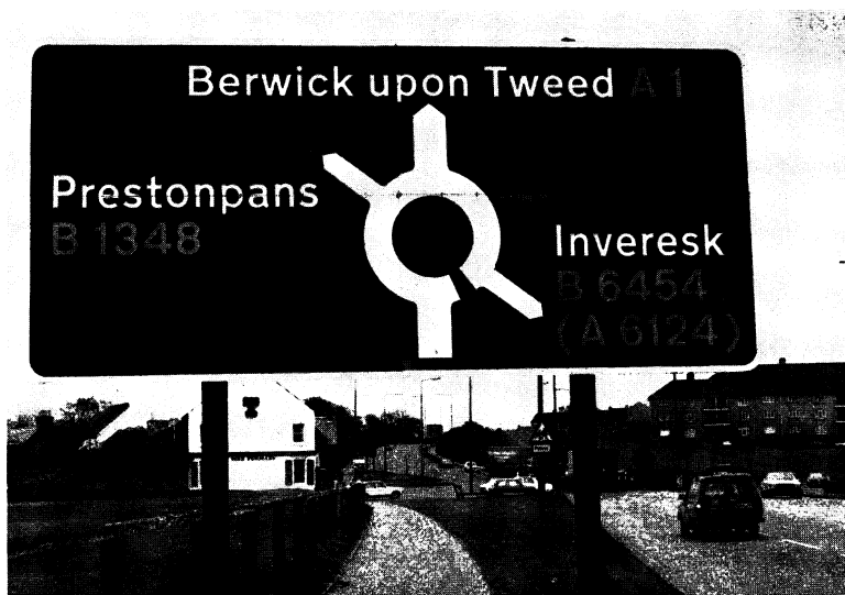
Figure 20. Scheme used in road signs to indicate required direction round a roundabout. Strictly, the depicted defect in the road is a lie, but the motorist understands what is required of him (photograph: John Wilkie)
