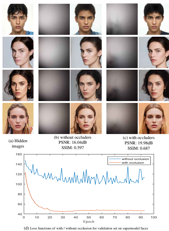
Fig. 13. The results of with and without partial occlusion on supermodel face reconstruction. (a) Hidden images. (b) Input and reconstruction results when there is no occlusion. (c) Input and reconstruction results when there is a partial occluder. In terms of quantitative comparison, the PSNRs of with and without occlusion are 16.04dB and 19.37dB, and SSIMs are 0.597 and 0.674, respectively. (d) Loss functions with/without partial occlusion. This shows that partial occlusion is helpful to NLOS-OT, proving that NLOS-OT has learned relevant knowledge about inverse light transport.
