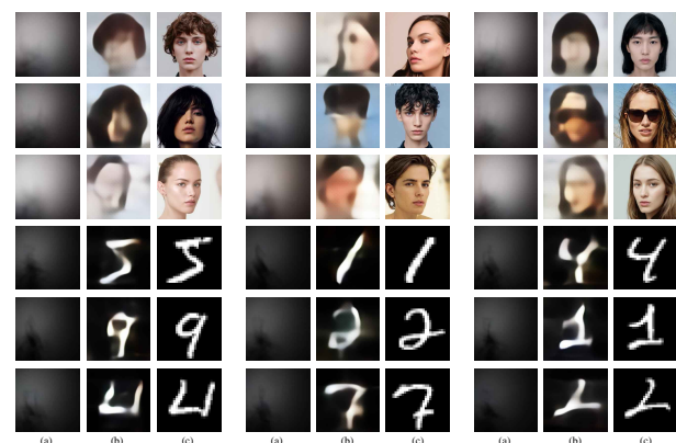
Fig. 7. Generalization of NLOS-OT model. When the dataset is complex, NLOS-OT has good generalization ability. The training set is STL-10, and the test set is MNIST and supermodel dataset. Left: input, middle: output, right: ground truth.
