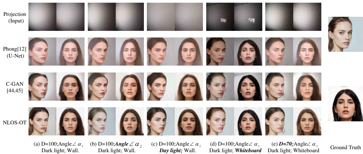
Fig. 6. Results under different optical transport conditions. With a specified target image, (a) illustrate the results of different methods under the optical transport condition: dark environment, distance D = 100 , angle \angle \alpha_1 , and the wall reflection. (b)-(e) represent the reconstruction results obtained by different methods after changing one of the four optical transport conditions in (a), respectively.
