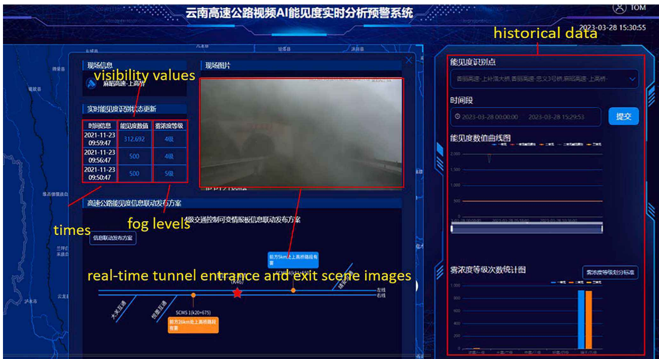
Fig. 13. The real-time visibility analysis and warning system interface based on video images for Yunnan Expressway.
