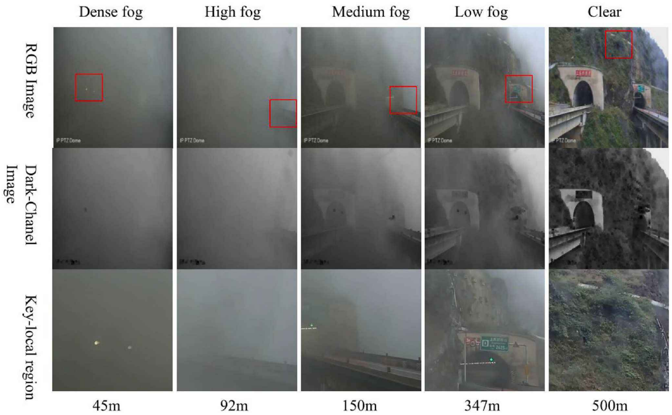
Fig. 3. Differences between dense fog and high fog images. The First line is the raw image in FEVI dataset. The red boxes show the main differences between the two types of images. The Second line is dark channel image. The third line is its corresponding key local region. The last line is the fog visibility value.
