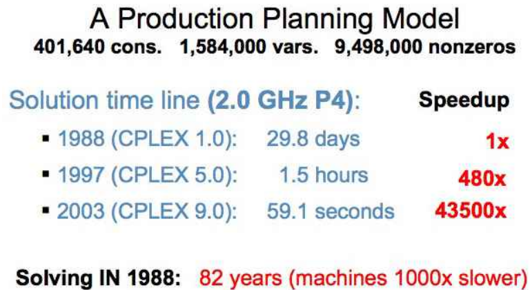
Figure 35: Martin Grötschel’s account of speedup in one production-planning problem. Reprinted from Grötschel (2009).
