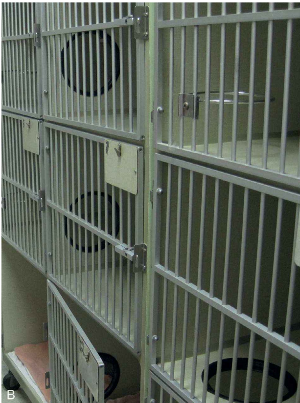
FIGURE 11-12 Some shelters and veterinary practices modify their cage banks by having a carpenter make an opening, or “pass-through,” between two smaller cages to create larger spaces with two separate compartments. One compartment can be used for feeding and the other for toileting. (Courtesy E. Sundahl)
