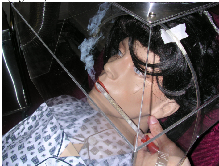
Figure 4 Smoke profile for the extraction hood.
