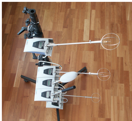
Figure 2 Thermal measurement station seen from above. Air velocity is measured at heights of 0.1 and 1.1 m, and operative temperature, air velocity and humidity are measured at 0.6 m above the floor.
