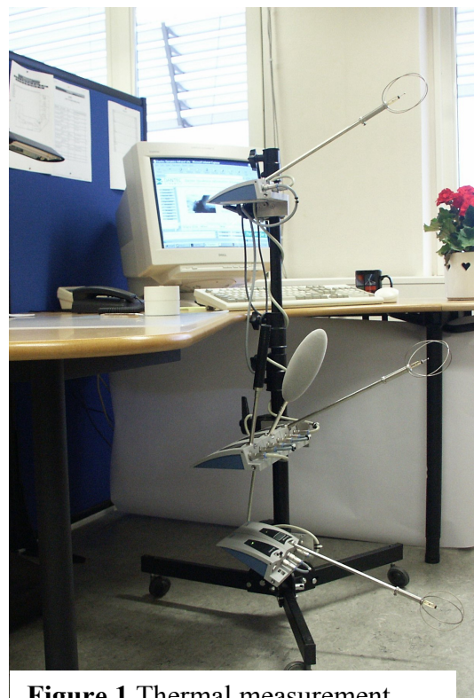
Figure 1 Thermal measurement station at work.
