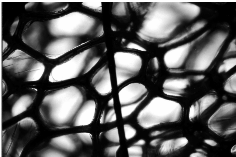
Figure 1 Photomicrograph of PUF at a magnification of 60 \times .
