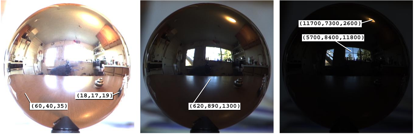
Figure 2: An omnidirectional radiance map This full dynamic range lighting environment was acquired by photographing a mirrored ball balanced on the cap of a pen sitting on a table. The environment contains natural, electric, and indirect light. The three views of this image adjusted to (a) +0 stops, (b) -3.5 stops, and (c) -7.0 stops show that the full dynamic range of the scene has been captured without saturation. As a result, the image usefully records the direction, color, and intensity of all forms of incident light.
