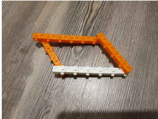
Figure 2: 4-Bar Linkage scewed to the left.
