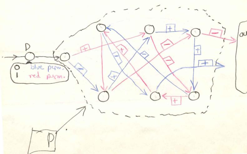
The cicles represent places where a digit can be stored. During each cycle either the red permutation of digits or the blue takes place. This is decided by the digit in D at the beginning of the cycle. The D digit moves to the first circle or storage place in P during the cycle after it has determined the choice of the permutation.
