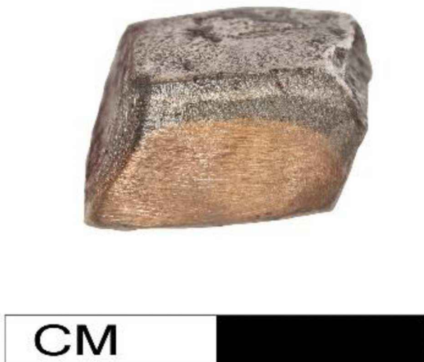
Fig. 5. A section of 'cut-ingot' with hidden Cu-rich core, courtesy of the Beth Shean Expedition.
