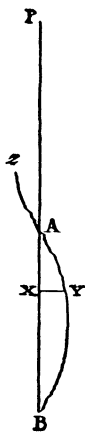
Figure 101. EULER'S device for bounding the buckling load of a heavy vertical column with pinned top (1778) 19-21
