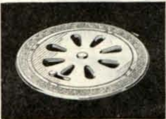
The artistic, polished aluminum registers (for front or rear compartments) have independent shutter controls.
