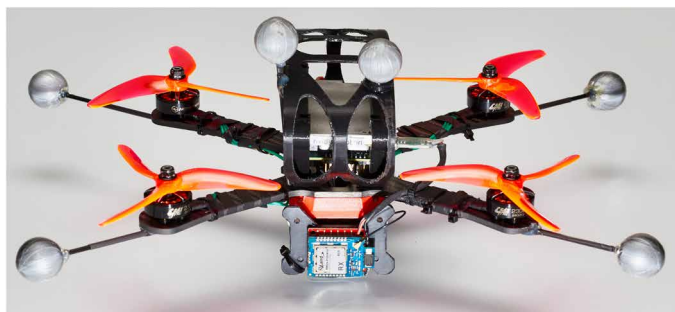
Fig. 2. The quadrotor vehicle. The autonomous platform used for the real-world experiments with a theoretical TWR of \sim 4 at 0.8-kg weight, equipped with a Jetson TX2, a Laird communication module, off-the-shelf drone racing components, and infrared-reflective markers for motion capture.
