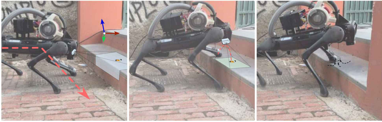
FIGURE 4 Snapshots and illustrations detailing the collection procedure. From left to right: The system first detects the cigarette butt (CB) using the front-facing camera, and afterward, the planner defines a new optimal pose for collection (highlighted in the first snapshot by the coordinate frame centered on the hip of the robot's leg associated with the collection mechanism) deviating from the predefined path shown in red. Once the robot reaches the collection area, it utilizes the down-facing camera to refine the previous estimate of the CB's location. Finally, the robot proceeds to perform the collection by stepping on the target and activating the suction. [Color figure can be viewed at wileyonlinelibrary.com ]
