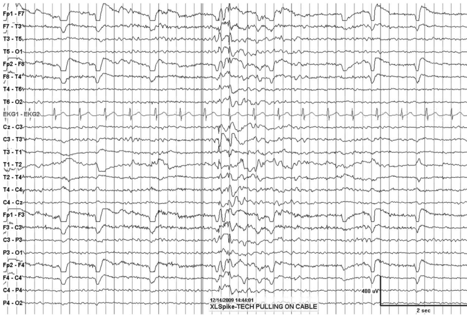
FIG. 10. Cable artifact incurred during transfer of the amplified multiplexed digital signal from the patient via cable telemetry to the epilepsy monitoring unit. Note the similarity to a burst of irregular generalized spike-and-wave discharge.
