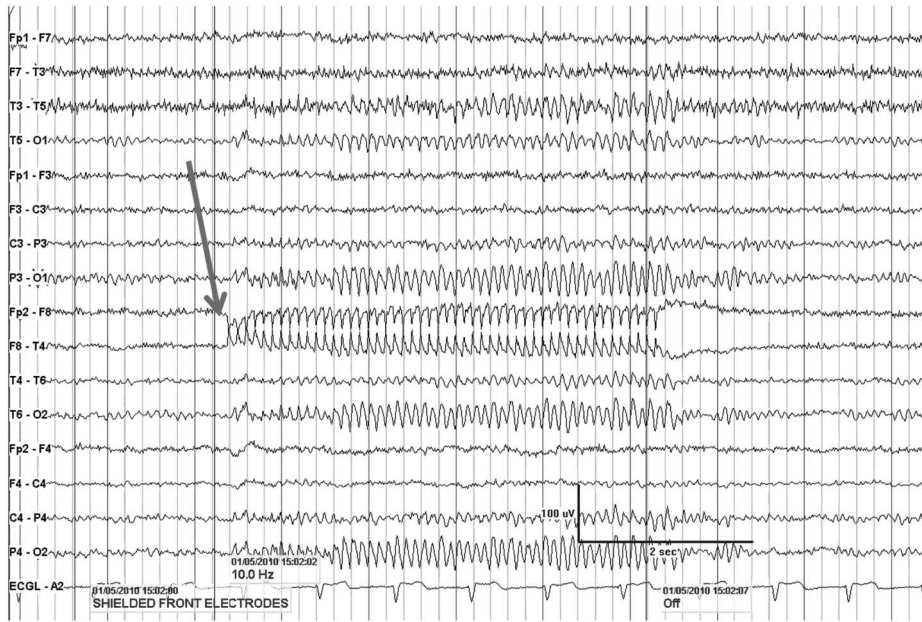
FIG. 6. A complex waveform simulating a focal seizure at F8 because of a single high-impedance electrode during intermittent photic stimulation. Intermittent “spikes” detected by the computer remitted after electrode reapplication.
