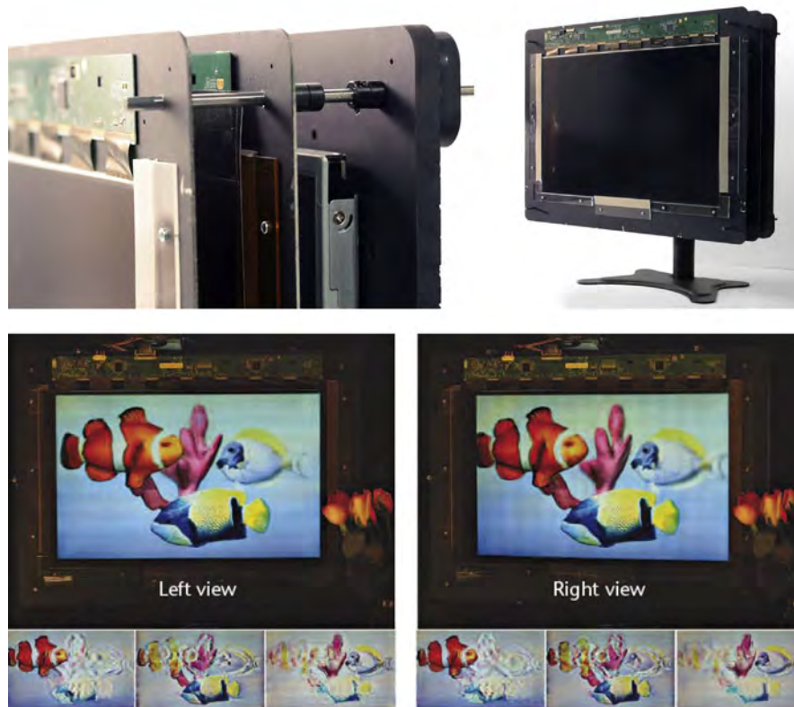
Fig. 26. Top row: a prototype tensor display. Middle row: two different views of a light field as seen on the tensor display. Bottom row: layered patterns for two different frames [297].
