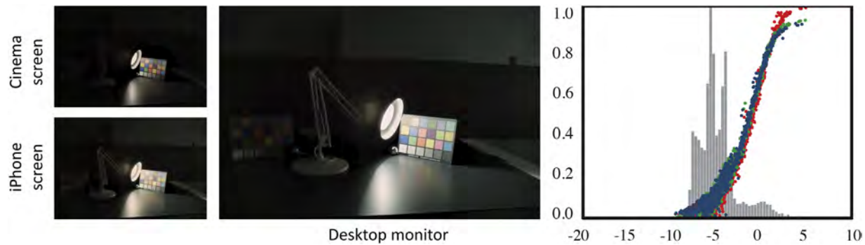
Fig. 13. Accurate color reproduction, taking into account both display type and viewing conditions (shown here for cinema screen, iPhone and a desktop monitor). The plot shows the image histogram in gray, as well as the input/output mapping of the three color channels [151] (image copyright ACM 2012). (For interpretation of the references to color in this figure caption, the reader is referred to the web version of this paper.)
