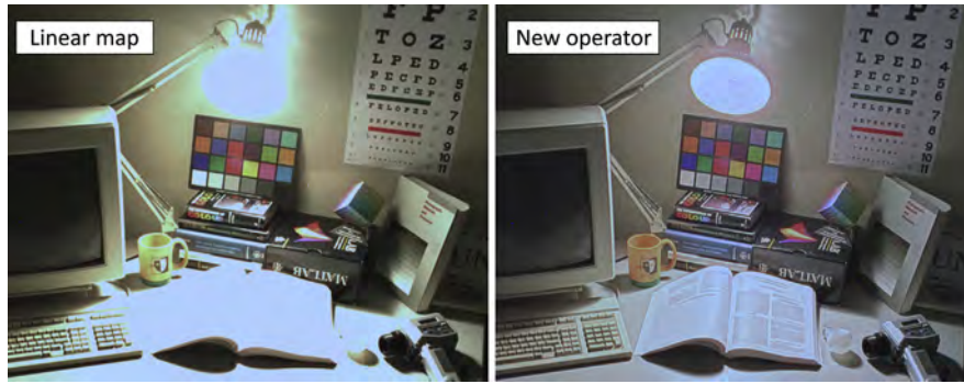
Fig. 7. Tone mapping allows for a better visualization of HDR images on displays with a limited dynamic range. Left, naive visualization with a simple linear scaling; right, the result of Reinhard's photographic tone reproduction technique [63] (image copyright ACM 2002). Radiance map courtesy of Cornell Program of Computer Graphics.
