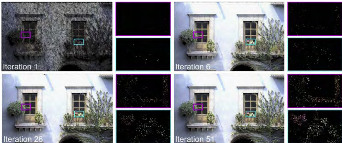
Fig. 27. Progressive reconstruction of a light field by adaptive image synthesis. In can be seen in the close-ups how the cumulative light field samples used represent a very sparse set of all plenoptic samples [311] (image copyright ACM 2013).
