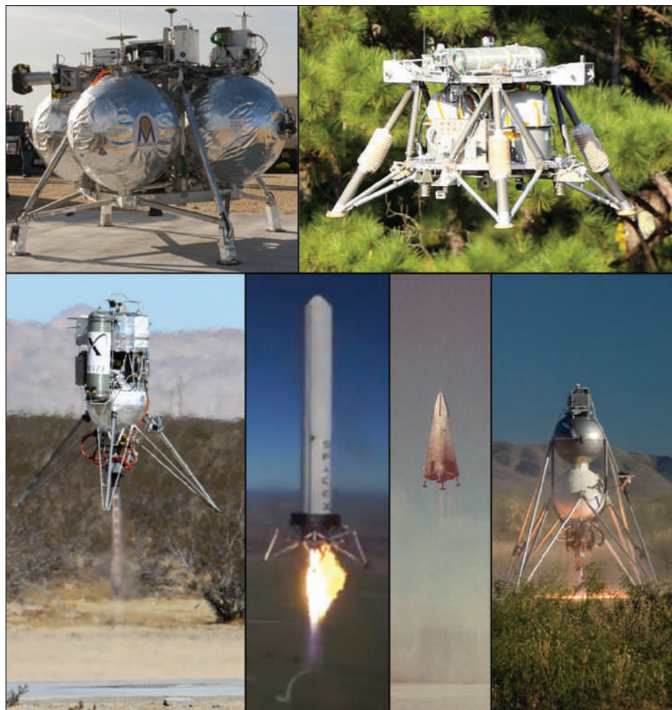
FIGURE 6 Various experimental vertical takeoff and landing testbeds. Clockwise from top left: NASA's Morpheus (left) and Mighty Eagle (right), Masten Aerospace's Xoie , SpaceX's Grasshopper , McDonnell Douglas' DC-X , and Armadillo Aerospace's Mod . Image credits: NASA/Dimitri Gerondidakis ( Morpheus ); NASA/MSFC/Todd Freestone ( Mighty Eagle ); Ian Kluff ( Xoie ); NASA ( DC-X ); Armadillo Aerospace/Matthew C. Ross ( Mod ).
