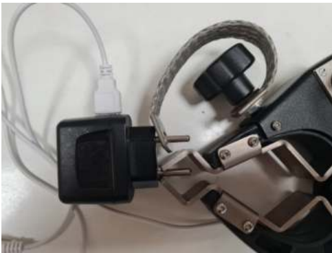
Fig. 5 Frequency response measurement of the charger's input plug.
