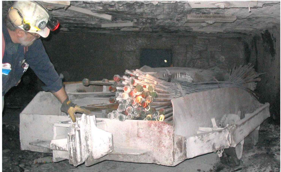
Fig. 10 Cable bolts stored on a mine car underground. These are 12-foot-long bolts that are being installed in 4-foot-high mine openings (photo by the author)
