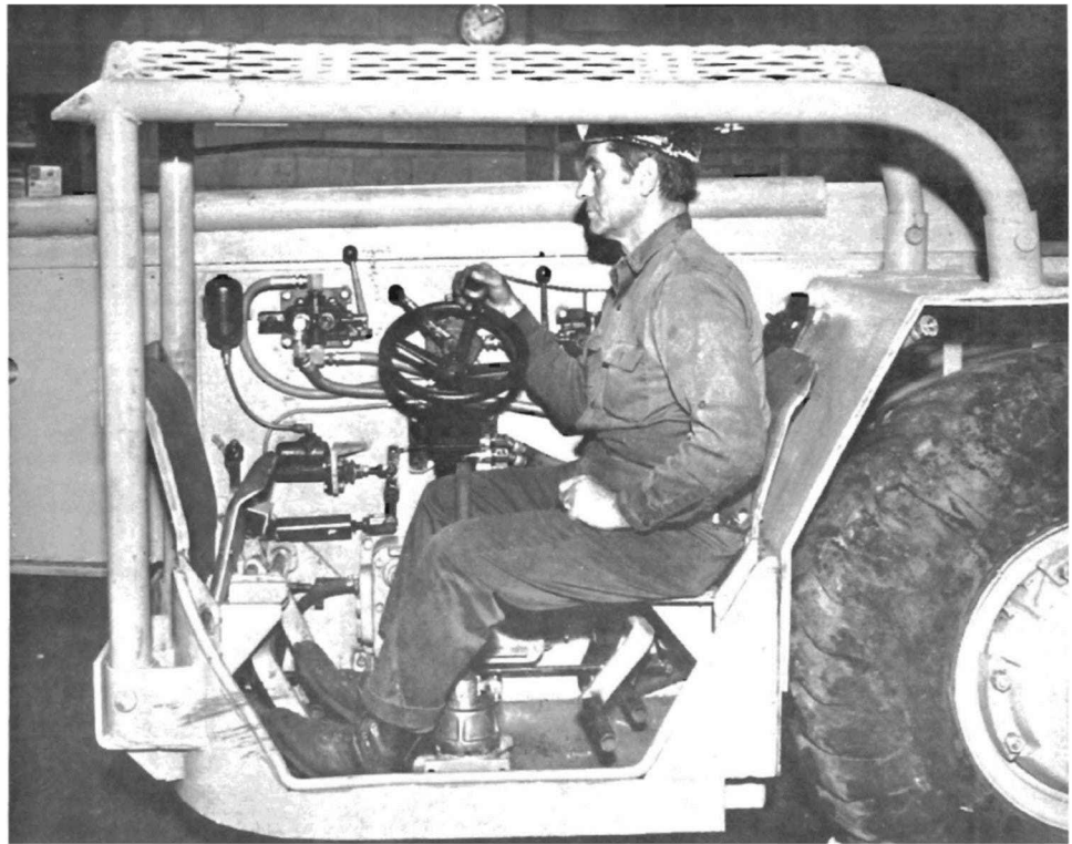
Fig. 4 An early retrofitted canopy installed on a shuttle car (source: US Bureau of Mines)
